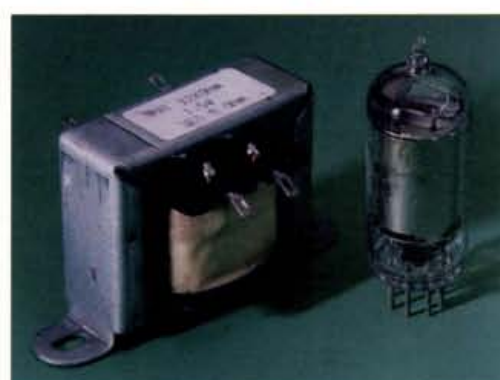
Fig. 4: The AOP-1 output transformer from Isoplethics matches almost perfectly to battery valved audio amplifiers.
