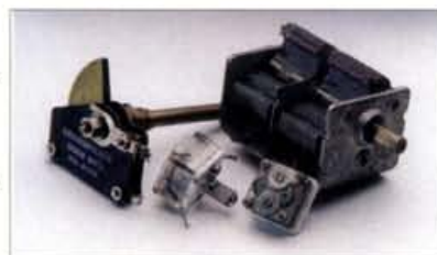
Fig. 3: Variable capacitors - particularly the 'open' air-spaced type are often available with trimmer capacitors (see text). If not, you can always incorporate low value type in parallel (see text).
