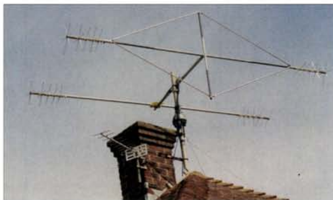
The antenna is mounted on a short mast on a KR-600RC rotator, which is fixed to the chimney using a double clamp. Some idea of the small size of the MQ-2 gain can be seen by comparison with the u.h.f. broadcast TV antenna.
