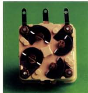
Fig. 2. Example of a miniature solid dielectric capacitor with fitted 'trimmers' (see text).
