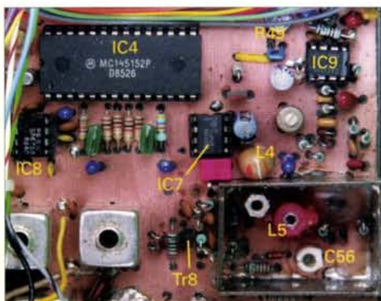
Close-up of the oscillator and modulator area of the 'main' board.
