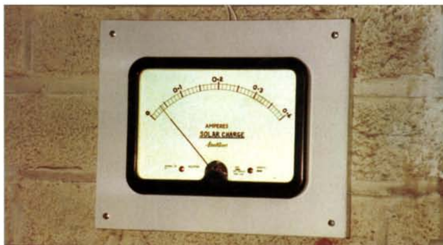
Fig. 2: Although not strictly necessary, being a Radio Amateur G4UBB fitted an ammeter so he could monitor the efficiency of the solar panel (see text).
