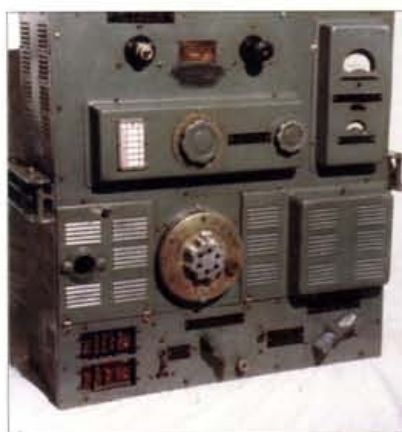
Fig. 1: The Saram 3-10 transmitter. The two doors either side of the large central tuning dial open to reveal the valves for the set.
