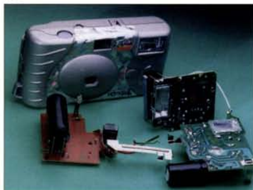
Fig. 1: Throw-away cameras can be a source of small electronic flash guns and high voltage capacitors. See text for more details.
