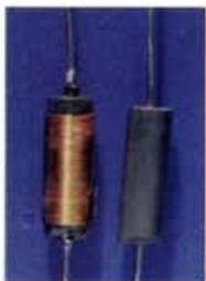
Fig. 7: Winding a 15µH choke on an Isoplethics IDCW5/16 powdered iron choke core is very easy and the results look good.
